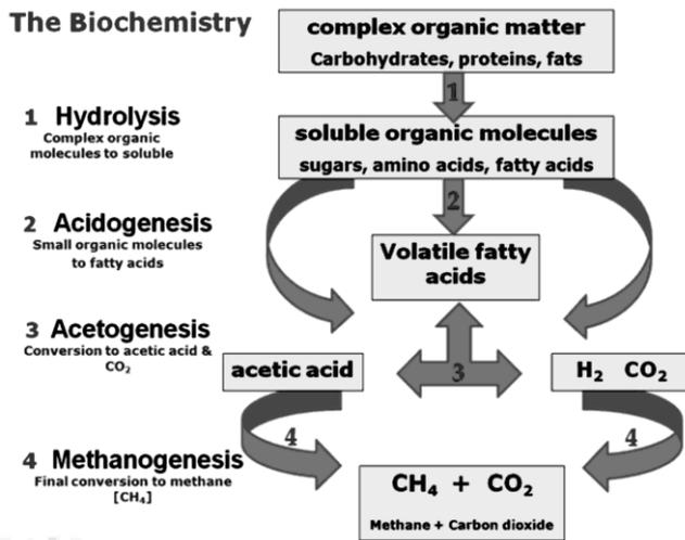
**Fig. 1: Schematic Representation of Anaerobic Biodegradation [18]**
